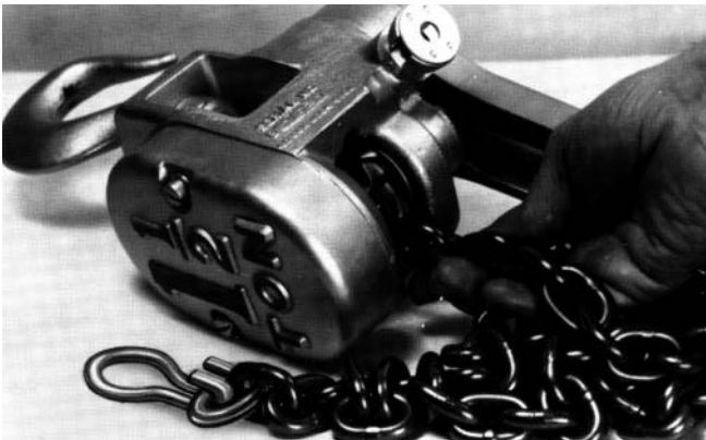
Figure 13. Chain Assembly - Hook End, 1 1/2 Ton
