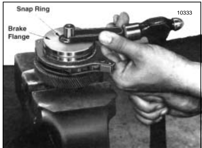
Figure 7-21. Removing Snap Ring from Load Brake Shaft
