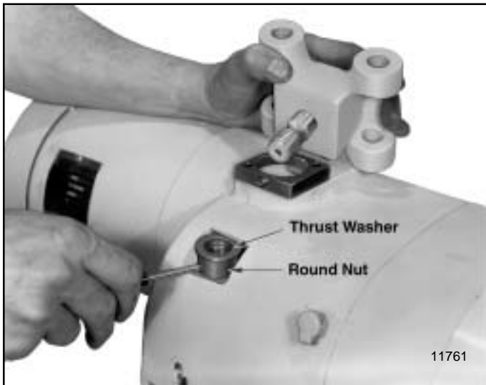
Figure 7-20. Removing Suspension Lug (1/4 thru 1 Ton Models)
