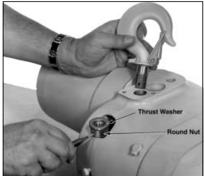
Figure 7-18. Removing Upper Hook and Hook Nut from Hoist Frame (1/4 thru 1 Ton Models)
