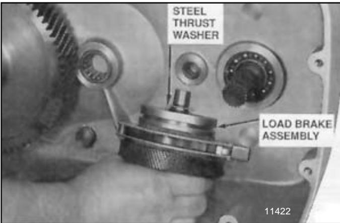
Figure 5-5. Removed Load Brake Assembly.
