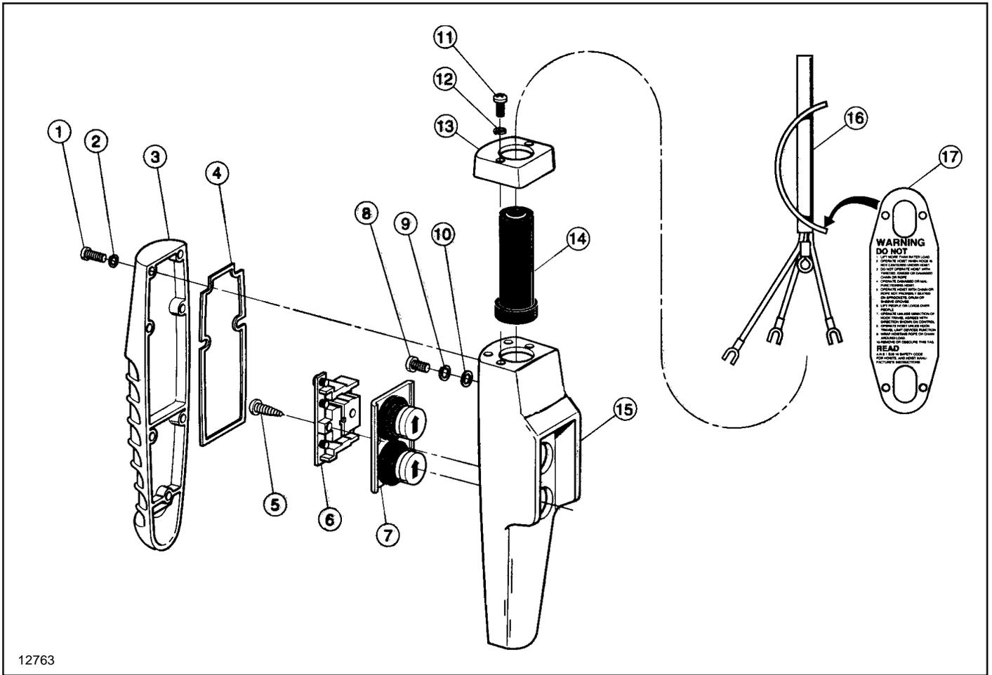
Figure 9-8. Push Button Station and Conductor Cable Assembly.
