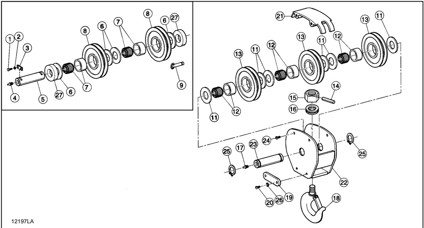
Figure 9-13. Upper and Lower Block Parts (3 & 5 Ton — Typical).
