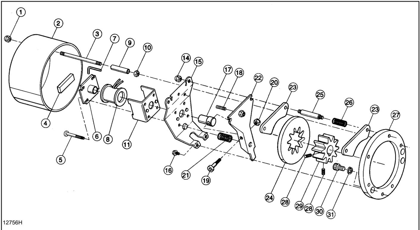
Figure 9-3. Hoist Motor Brake - Later Version.
