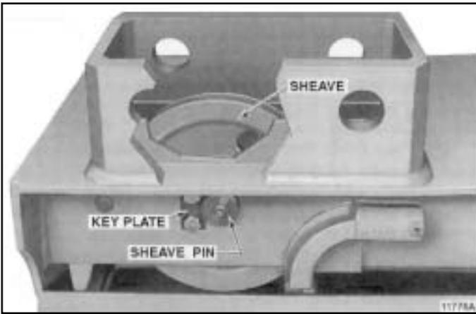
Figure 5-13. Upper Sheave Installed.
