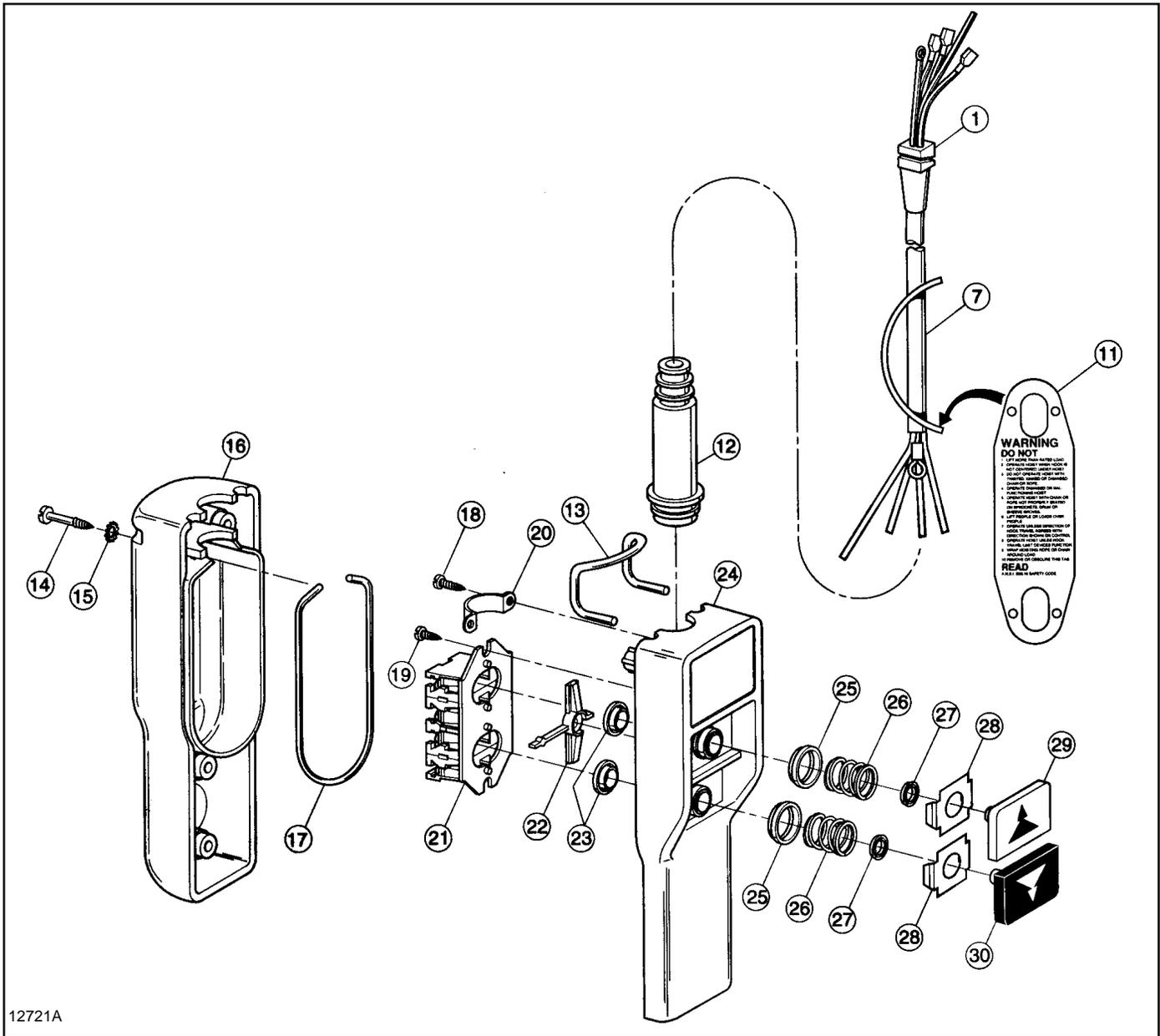
Figure 9-9. Push Button Station and Conductor Cable Assembly.
