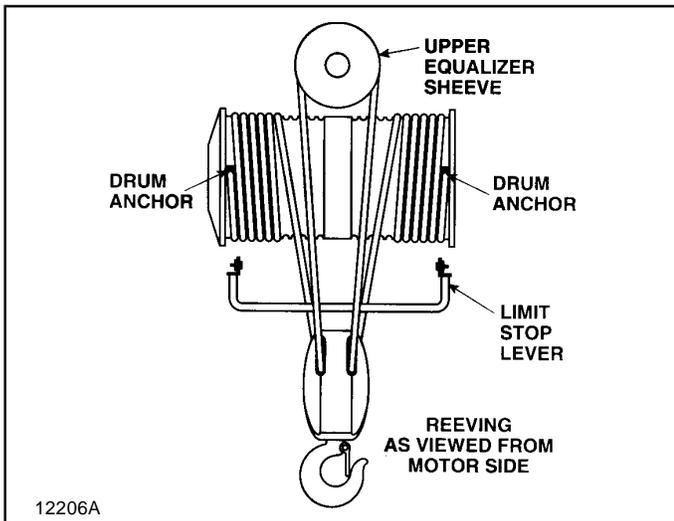
Figure 5-17. Hoist Reeving — Two Part Double.
