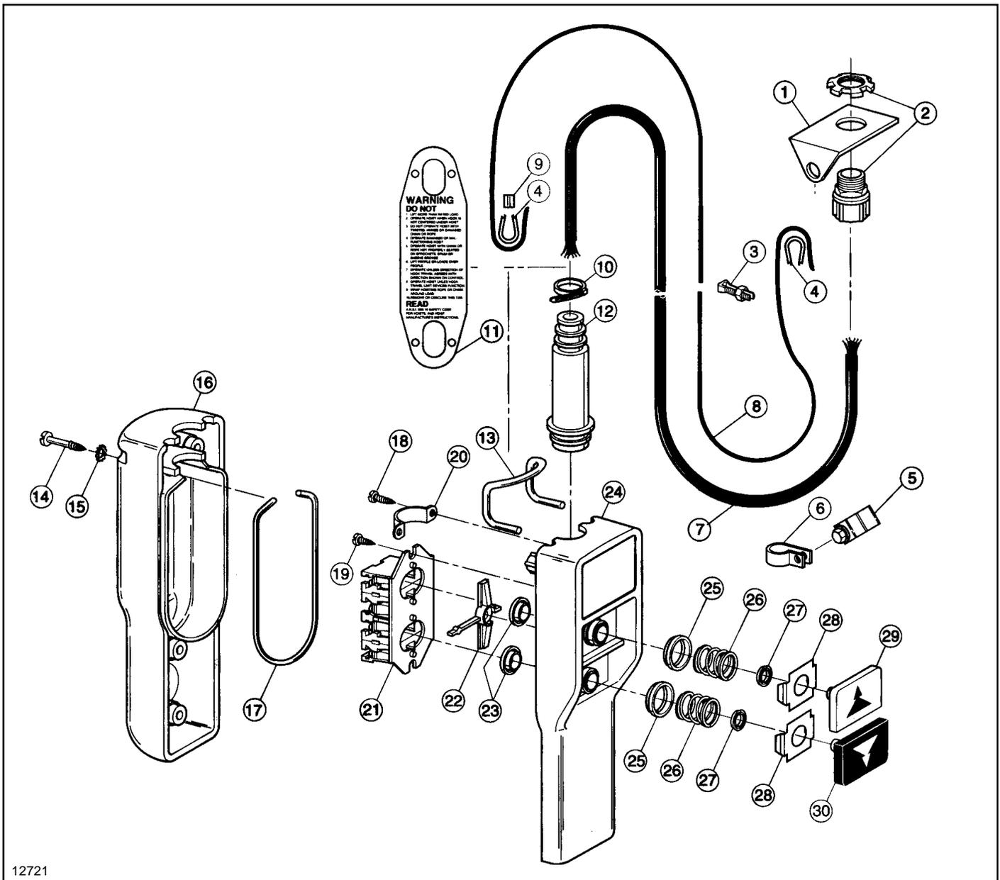
Figure 9-10. Push Button Station and Conductor Cable Assembly.
