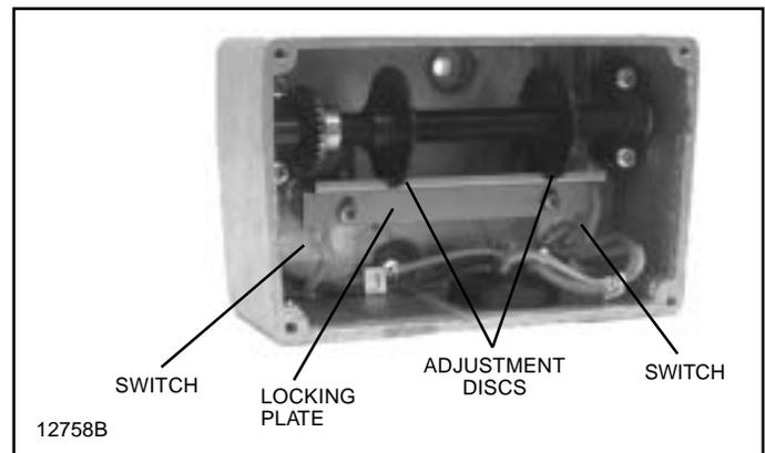
Figure 7-2. Screw-Type Limit Switch Adjustment.
