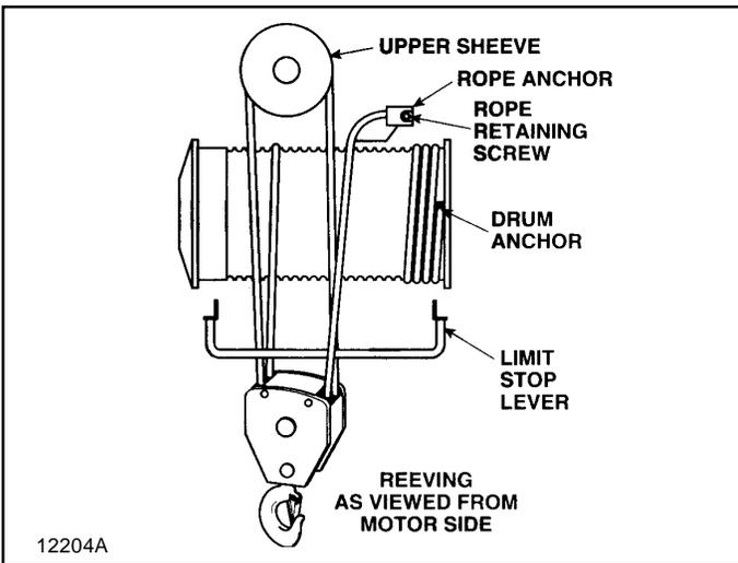
Figure 5-14. Hoist Reeving — Four Part Single.
