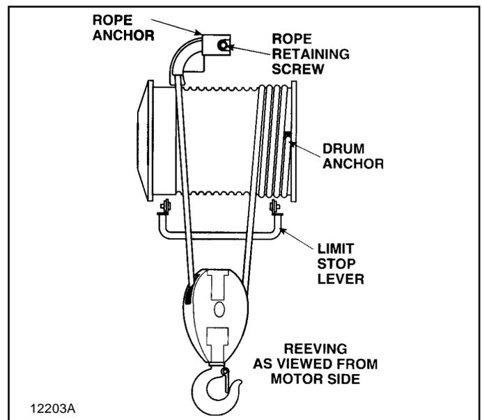
Figure 5-12. Hoist Reeving — Two Part Single.
