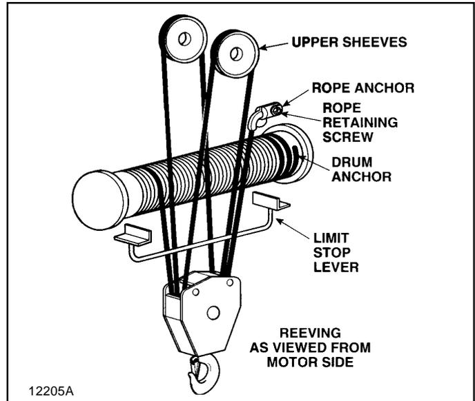
Figure 5-15. Hoist Reeving — Six Part Single.
