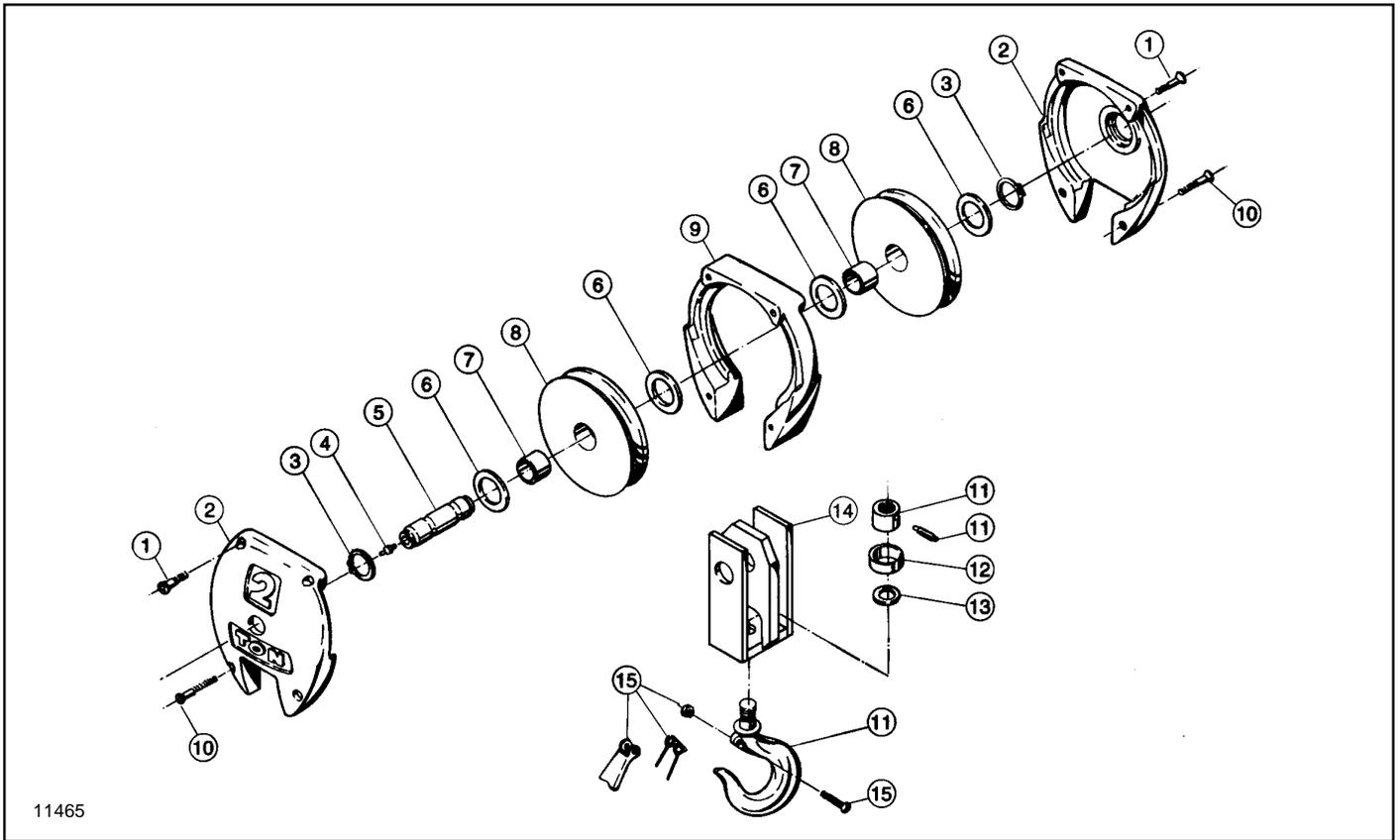
Figure 9-12. Lower Block Assembly—Two Parts Double Reeved.
