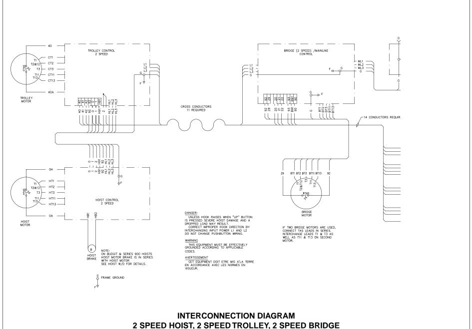
2 SPEED HOIST, 2 SPEED TROLLEY, 2 SPEED BRIDGE **PUSHBUTTON FROM BRIDGE**
