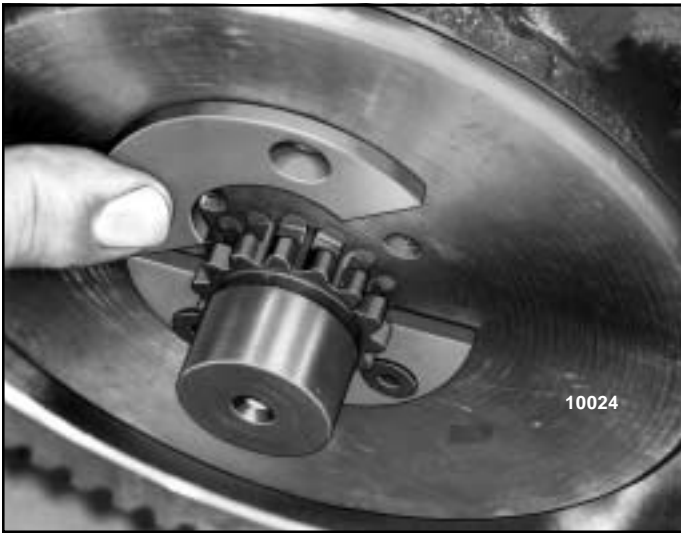
Figure 5-5. Installing Retainer Plates on Load Brake Shaft
