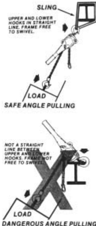
**Figure 4 - Pulling at an Angle**
